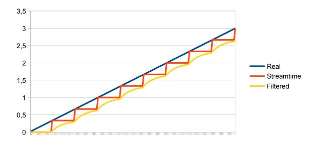
Figure 15.1: Low-pass filtered time values
